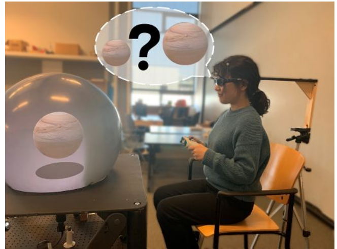
Figure 1. A user interacting with the Spherical Fish Tank VR display while performing the 3D perception task by judging the size of a virtual ball. The virtual ball looks smaller as user gets closer to the screen.
